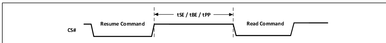
Figure-72. Program Resume and Erase Resume Sequence Diagram
